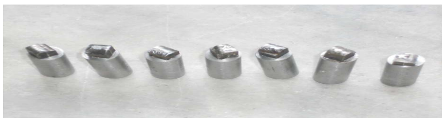
Fig. 12. Pin type samples for wear testing
